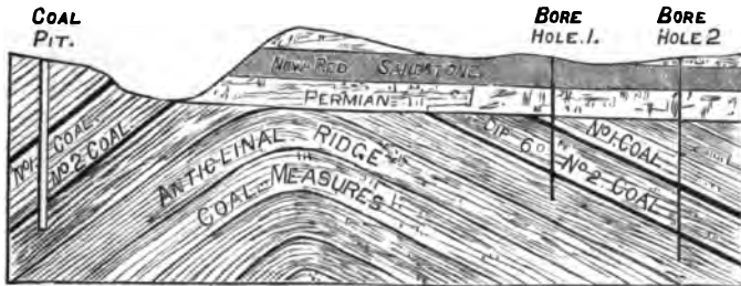
FIG. 61.—Section showing an anticlinal ridge, and eastward extension of coal-field entirely concealed by new formations, and only discoverable by boring.
